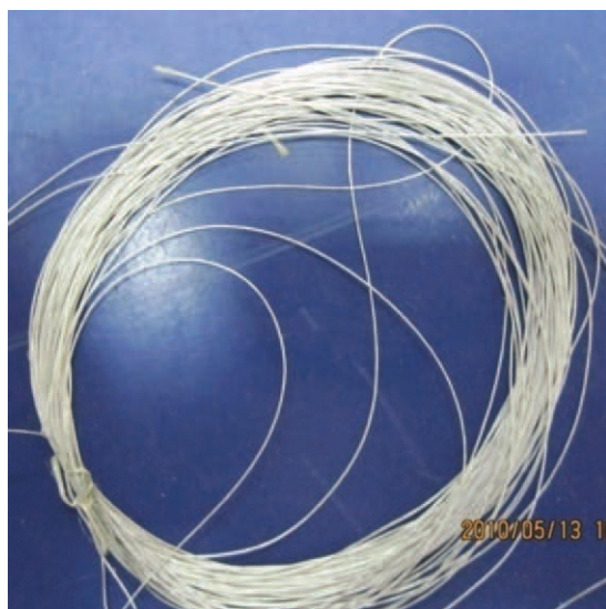
Figure 11 Appearance of silver deposits on para -aramid fibers. [Color figure can be viewed in the online issue, which is available at wileyonlinelibrary.com .]
